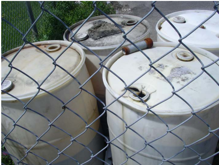
Figure 4-16: Automobile Repair Facility (HSI-A-506) With Unlabeled and Unsealed 55-Gallon Drums
