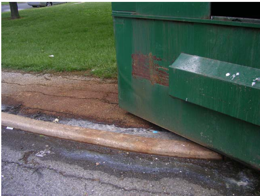
Figure 4-63: A Leaking Dumpster at ISI-A-1537
